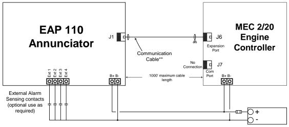
\*\*8 conductor Shielded Twisted Cable c/w RJ45 connectors. Communication cable wiring must be suitably routed to protect it from sources of electrical interference. Refer to section 2.4. of this manual for further information.
